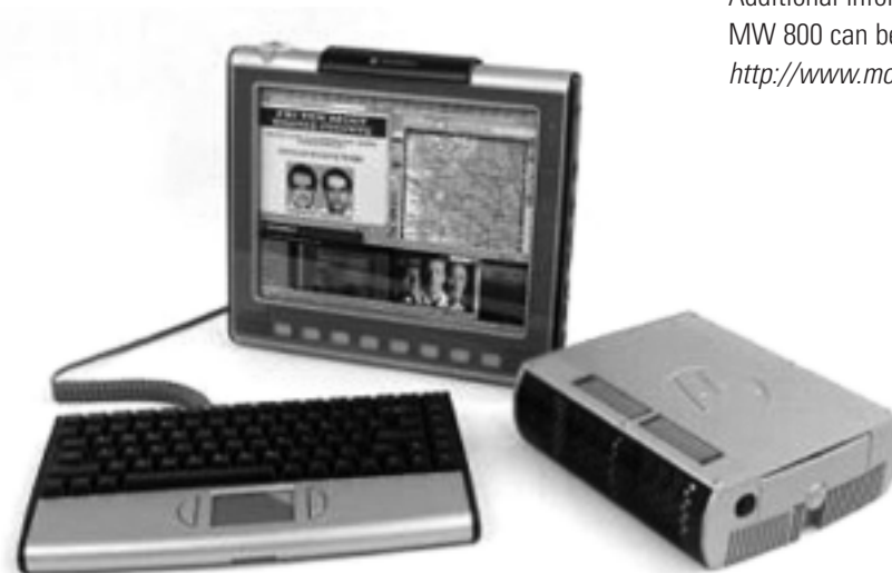
The MW 800 Display and Keyboard pictured with the Central Processing Unit (CPU)
